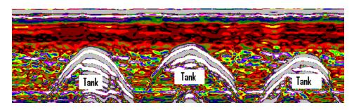
Geophysical methods can provide a cost effective means to screen a site and identify the location of USTs.
