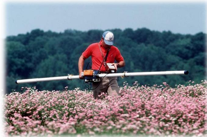
Geophysics provides a non-destructive, non-intrusive assessment of site conditions. Geophysics can be performed in areas of sensitive environmental conditions such as wetlands. A geophysical assessment can be much more cost effective than a haphazard excavation program and an uncertain restoration.
